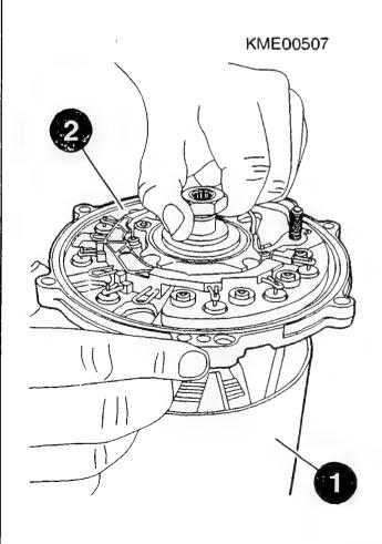
Dismantling windingless rotor
